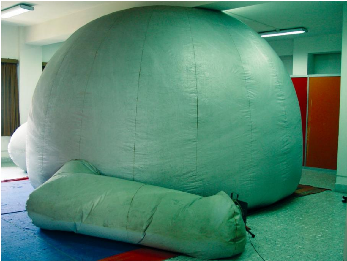
Pic 4: Air flow from Fan to Inflated Dome
