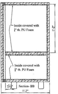
Note:- Box made with  $\frac{1}{2}$ " Phenol bonded ply. All out sides to be covered with rexin (apprived colour).
