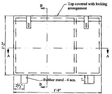
Note:- Box made with  $\frac{1}{2}$ " Phenol bonded ply.
